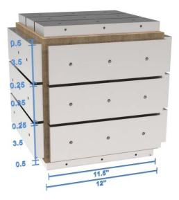
Figure 2. Loading plates on cubical specimens
