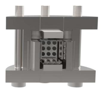
Figure 3. Cross-sectional view of RPS-600 Polyaxial cell
