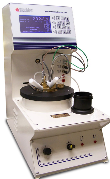
Flash Point by Automatic Abel Flash Point Tester
